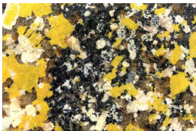
Fig. 9 Stained slab (4 × 8 cm) of a schlieren showing strong modal and grain-size asymmetry (Spec. VH3-7B). The asymmetry is clearly shown by stained alkali feldspar. The finest-grained zone is about 1 cm thick and essentially lacks alkali feldspar. This zone is in sharp contact with cg granite on the left . The first occurrences of alkali feldspar to the right are much finer grained and coarsen to the right
